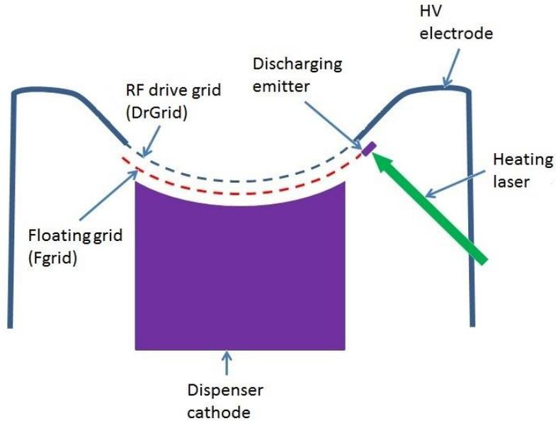
The floating grid can aid in the suppression of cathode arcing in the vacuum electron device.
