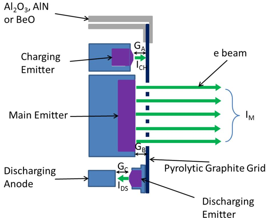
A floating grid thermionic cathode
