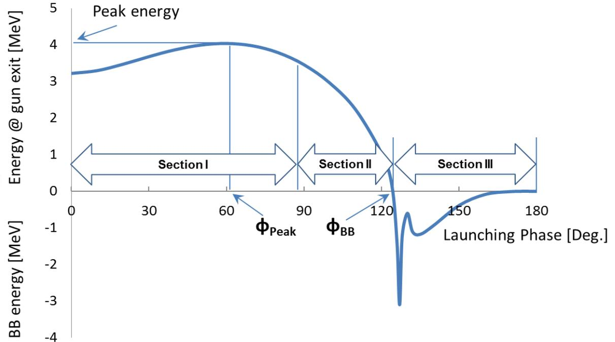
Electron energy at gun exit or back-bombardment (BB) energy vs. cathode launching phase (initial phase).
