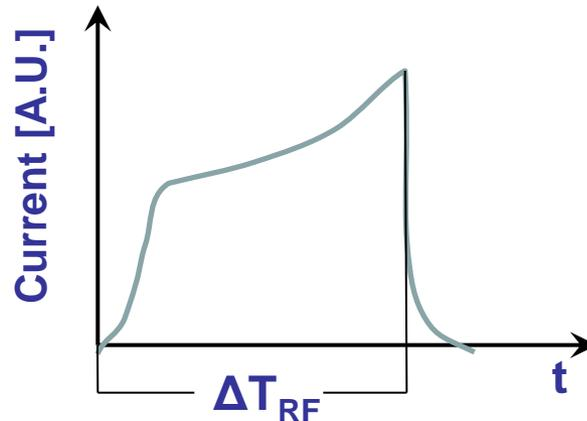
Output current signal from a thermionic RF gun
