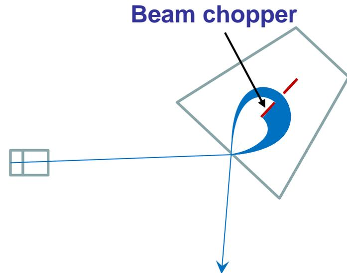
$\alpha$  magnet for suppressing section II beam.
